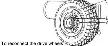
Turn the drive collar (part "A") until it reconnects with the wheel and then move the trolley until the collar connects with the drive.
