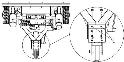
Fix the support arms onto back wheel frame as per illustration.
