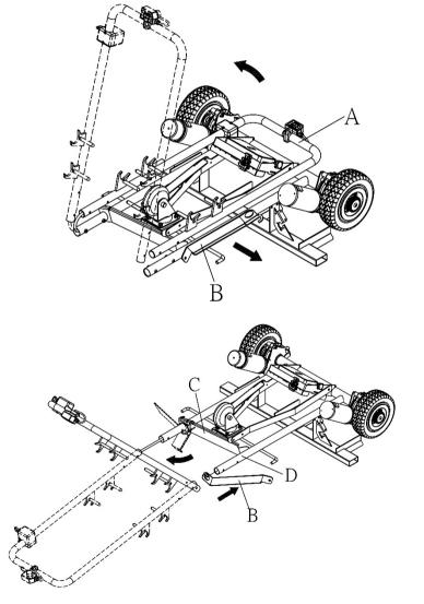
Insert support arm "B" onto the shaft base in the direction of arrow.
