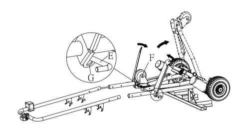
Pull up wheel "F" & frame as per arrow direction. Swing support arm C & B as per illustration and lock groove "G" Onto cross bar "E". Ensure that the groove is locked onto bar "E".
