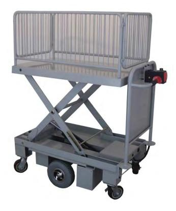
Centre Drive Cagemate Trolley with Push Button Lift and Drive with Removable Cage Sides
