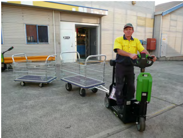
The T1000 Platform Tug towing HG-513 Mesh Basket Trolleys with Optional Tow Bars and optional 250mm Puncture Proof Pneu' Castors
