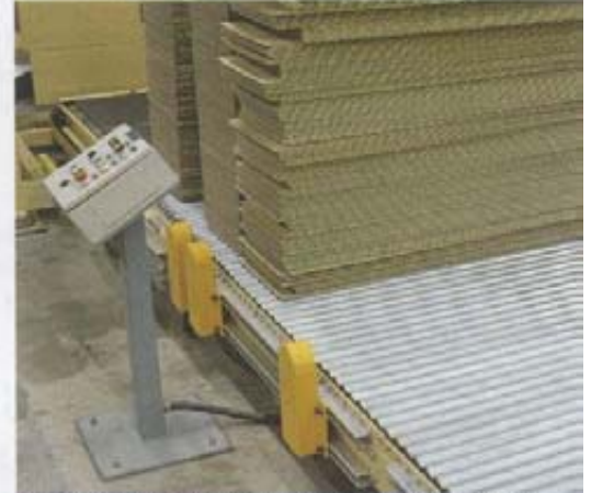
HEAVY DUTY BELT UNDER ROLLER ACCUMULATING CONVEYOR
