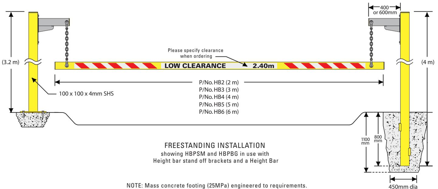
NOTE: Mass concrete footing (25MPa) engineered to requirements.
