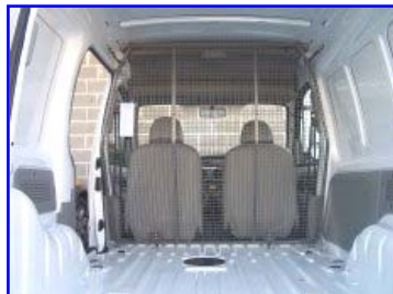
Mesh barriers for the larger vehicles
