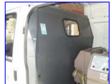
Barriers have a full frame and standard brackets for extra safety
