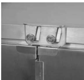
J clip to hold doors closed during transit
