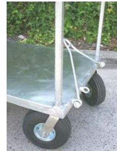
Loose towing device
