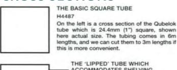
ACCOMMODATES SHELVING The 'lipped' tubing, also shown here actual size, is used for the inset of glass or perspex. Turned the other way up it allows the inset of timber or particle board.
