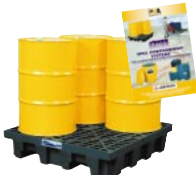
4-DRUM SQUARE PALLET CAT. NO. 28254 Sump Capacity: 250 Litre / Load Bearing Capacity: 2268 kg 2, 3 & 4 Drum In-line available 8 Drum Accumulation Centre also available
