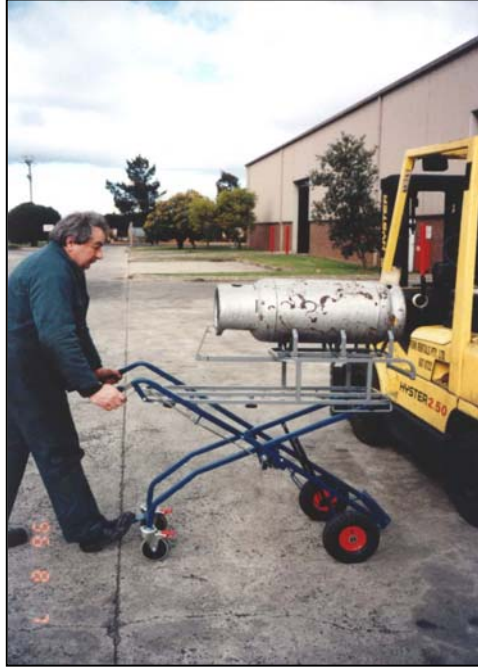
Lay unit flat, release FlexiLift latch and allow cradle to rise on gas struts to horizontal position.
