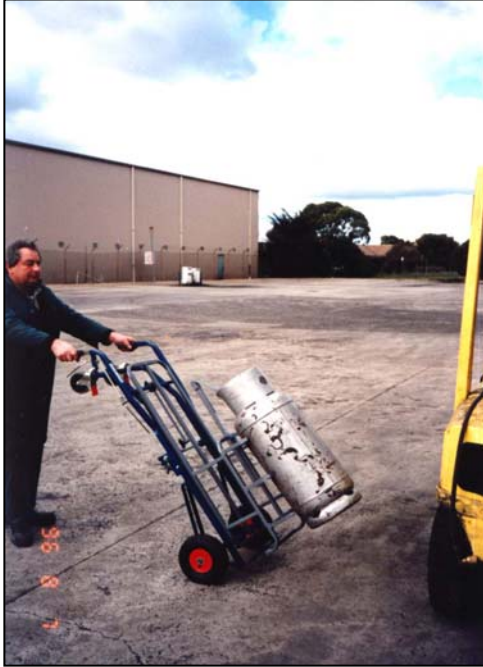
Wheel up to Gas Bottle and attach to cradle using cradle strap.
