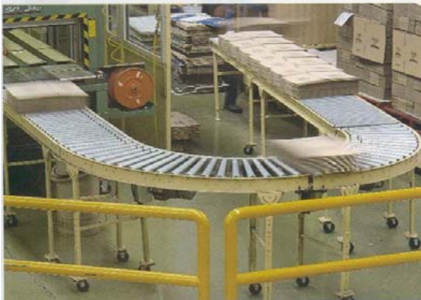
TYPICAL XENEROL LINESHAFT CONVEYOR WITH TRUE TAPER ROLLERS IN THE CURVES
