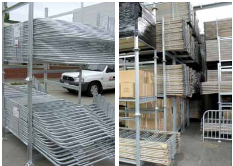
EFS – Stillages make storage and handling of panels simple and space efficient.
