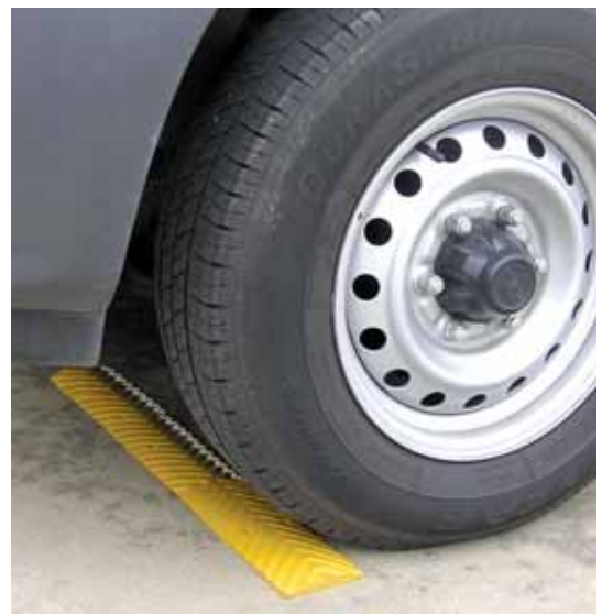
Rumble strip – a speed moderator or lane divider.
