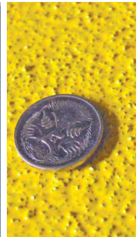
Diamond hard silicon-carbide aggregate in epoxy resin.
